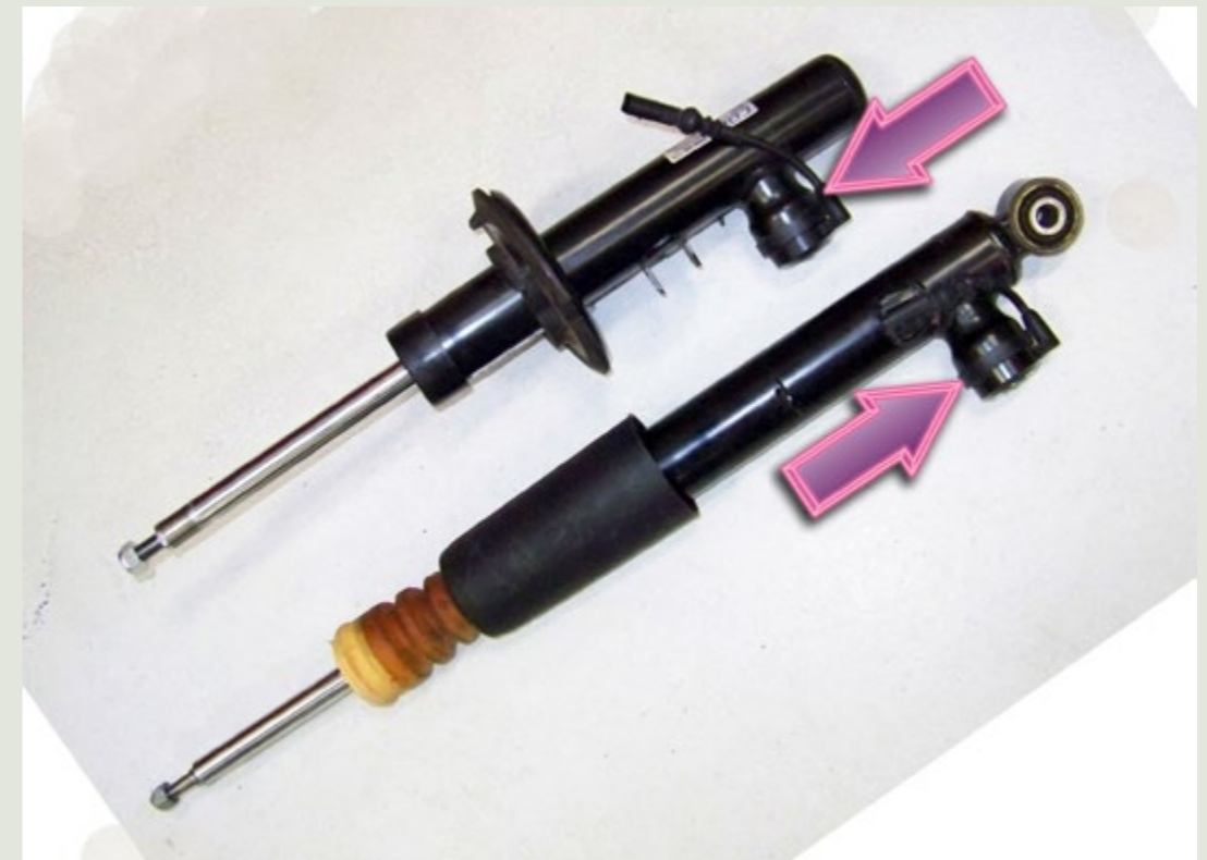
Audi OEM shocks have actuators that change damper valving, on command. Electronic Damping Cancellation Kit resistors modify circuit voltage to satisfy the control unit, and keep the dash light off. ES2608438
